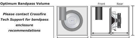
Note: Dimensions for recommended enclosure are with consideration of using .75" (19mm) MDF board. Be sure to add .050ft3/1.42L for driver displacement as well as the volume of the port to all enclosures, except for the optimum recommendation as those dimensions already include woofer displacement but DO NOT include port displacement.
