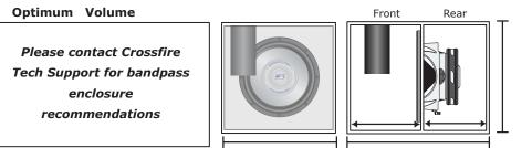
Note: Dimensions for recommended enclosure are with consideration of using .75" (19mm) MDF board. Be sure to add .050ft3/1.42L for driver displacement as well as the volume of the port to all enclosures. except for the optimum recommendation as those dimensions already include woofer displacement but DO NOT include port displacement.
