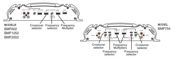
On the two channel amplifiers only is another crossover section with a selector switch marked HPF/FULL/LPF. This crossover section is designated to the preamp output. The crossover frequency is selected by the crossover allocated for the amplifier itself, however can be used in Highpass, Lowpass, or Fullrange independently of that crossover. This allows for multiple system configurations to be made.
